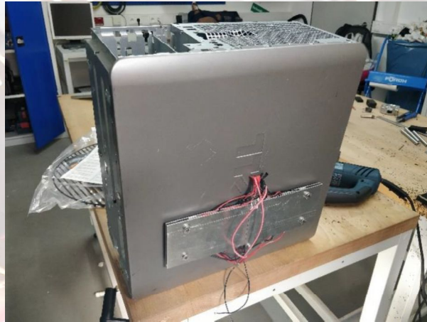
Figure 13: Mounted Peltier elements on the case
