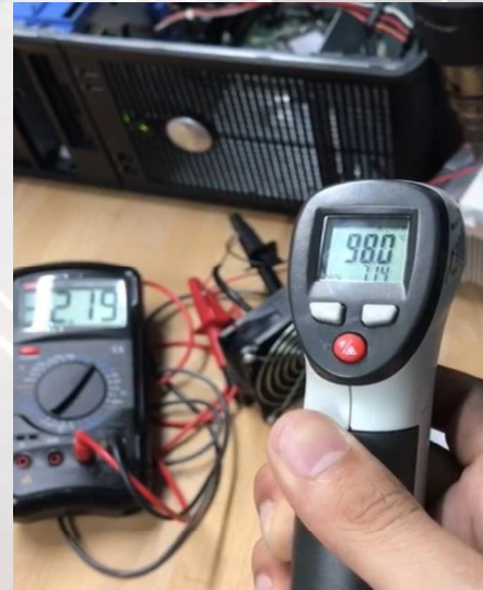
Figure 4: Measurement with a heat gun
