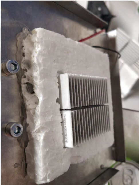
Figure 11: Ice on the surface of the heatsink
